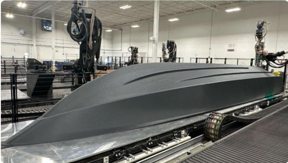
Robotic arms 3D print drone boat
